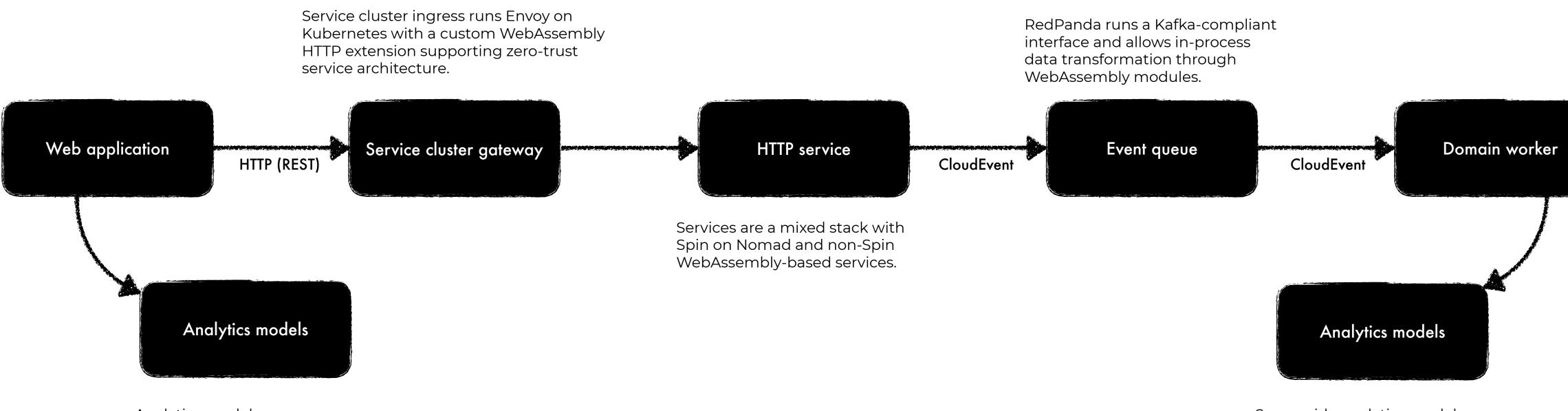
Analytics models are statistical algorithms built as WebAssembly modules Server-side analytics models are identical to the browser-based models enabling complete re-use.
